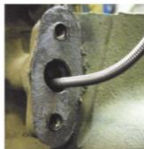
2 Attach flexible bit to drill, insert tip into port
